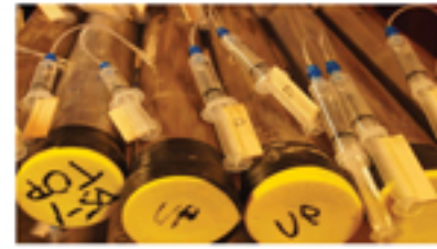
Fig. 4. Pore water sampling from the Lake Vättern sediment cores
