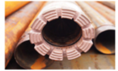
Fig. 3. Bore crown with core catcher inside
