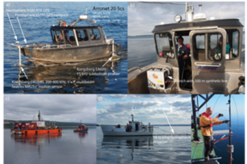
Photos of field work in Lake Vättern: a, b) RV Skidbladner equipped with a multi-beam echosounder and subbottom profiler (see photo for technical specification). RV Skidbladner is the Department of Geological Science's 6.4 m long aluminum boat made in Sweden by Arronet ( http://www.arronet.se/ ). It has been specifically outfitted for high-resolution geophysical surveys in lakes and near shore areas. c) The floating barge used by the company Asera Mining to drill into the bedrock of southern Lake Vättern for mine prospecting purposes. The sediment coring system we adopted when using this platform consisted of tools added to an HQ wire line drilling system, including HQ-3 plastic liners (inner diameter of 63 mm) for collection of unconsolidated sediment. In total, we core through the upper 70 m of unconsolidated sediments. d) Seismic reflection profiling was carried out with a 0.3 l (20 cu in) Bolt PAR airgun and 18 m long hydrophone streamer. This was done with the 10 m long vessel Hamnen. d) Piston coring of the uppermost 6 m of the sediment stratigraphy from Asera Mining's drilling platform.
