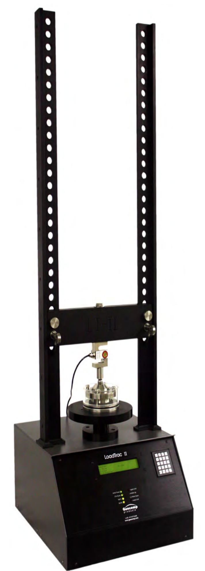
Figure 7. Automated incremental load and constant rate of strain consolidation system at IGV, Stockholm University. Manufactured by Geocomp Corporation, Acton, MA, USA. The load frame has a 44 kN (10,000 lbf) capacity, allowing applied loads of up to 20 MPa on standard 5 cm diameter (2 cm thick) samples. This equates to in-situ pressures at burial depths of > 2 km below the seafloor.
