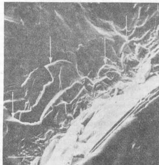
Fig 4. SEM photograph of replica surface of mechanically ruptured edges on a quartz flake. Scale: 70 \mu m. From Knutsson 1988a, fig 67.
